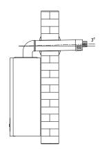
Figure 20 Condensing boiler flue slope
