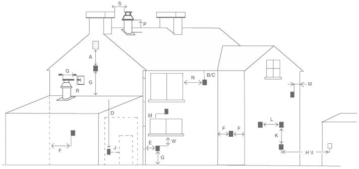
Figure 16 Environmental locations of flue
