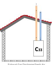
Exhaust Gas Discharge Fresh Air Intake with Split Flue Sets
