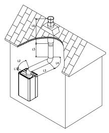
Figure 25 Vertical flue set installation
