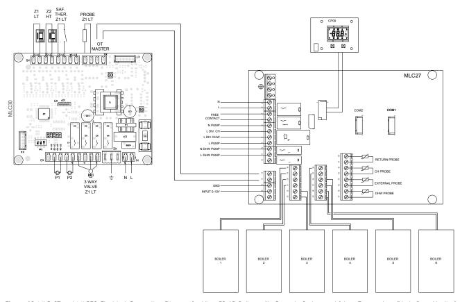
Figure 40 MLC 27 and MLC30 Electrical Connection Diagram for Viwa 50-65 Boilers with Cascade System and 1 Low Temperature (Underfloor Heating) Zone System
