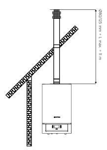
Figure 24 Vertical flue set installation
