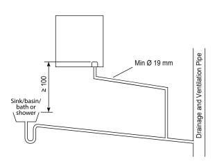
**Figure 31** Connection of Condensate Water Drainage Pipe at Indoor Bathroom Drainage Lower Level
