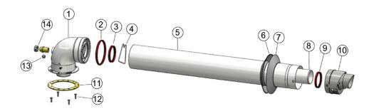
Figure 17  $\varnothing$  80/125 mm Concentric Flue Set
