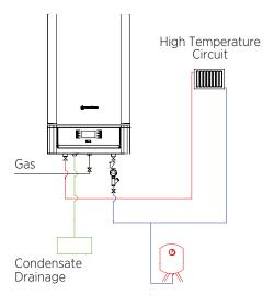
Figure 29 Connection Diagram of Single Boiler and 1 High Temperature Circuit
