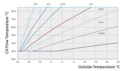
Figure 45 Outside Temperature Sensor Curvex
