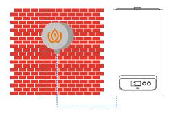
Figure 44 Outside Temperature Sensor
