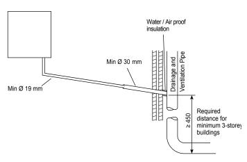
Figure 34 Connection of Condensate Drainage to Drainage and Ventilation Pipe
