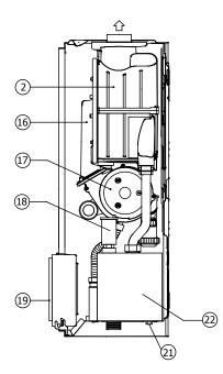
Figure 41 Components of the Boiler
