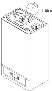
Figure 8 Filling the condensation flusher
