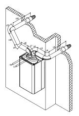
Şekil 26 Example of Split Flue (Hermetic) Type
