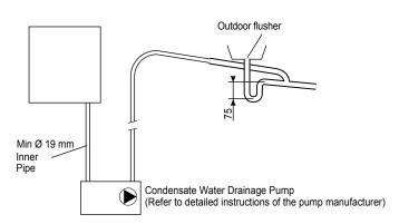
**Figure 33** Typical Connection Method of a Condensate Water Drainage Pipe (refer to detailed instructions of the pump manufacturer)
