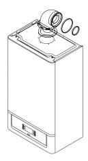
Figure 24 Vertical flue set installation
