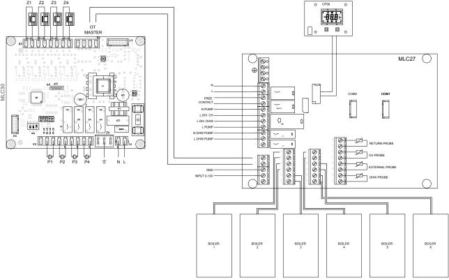
Figure 39 MLC 27 and MLC30 Electrical Connection Diagram for Viwa 50-65 Boilers with Cascade System and 4 High Temperature (Radiator) Zone System
