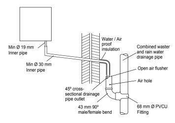
Figure 35 Connection of Condensate Drainage to Rain Water Drainage
