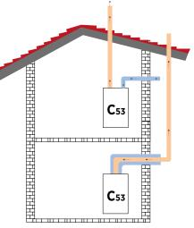
Exhaust gas discharge and fresh air intake with concentric flue kit and split flue kits
